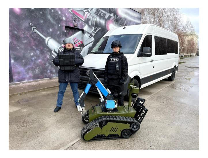
The control of the robotic complex is carried out both by cable and by radio, depending on situation. The duration of continuous operation of the robot is from two to four hours. The caterpillar platform allows Zirhli Tulpor to overcome thresholds 250 mm high and water barriers up to 200 mm deep.
